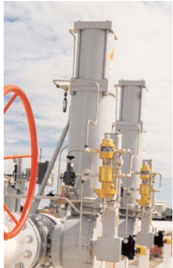
Figure 9.0 - Model HPP-SB Positioners on RPSR Actuators Becker Model HPP-SB Positioner on Ball Valve Regulators equipped with RPSR Actuators. HPP-SB Positioners feature high flow capacity, vibration resistance, and superior sensitivity. These features make it ideal for applications such as power plant pressure control – shown here. Additionally, the HPP-SB exhibits zero bleed at steady state, full-open and full-closed positions.
