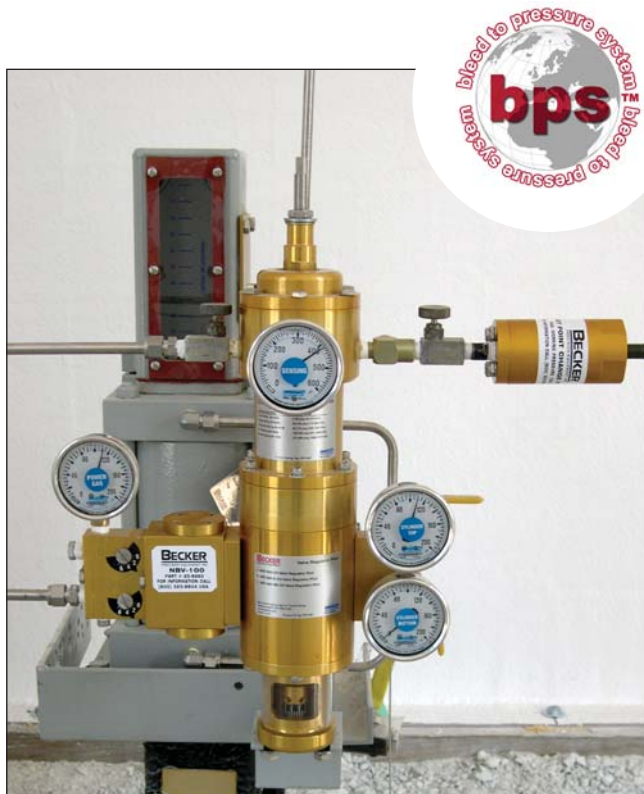
Figure 3.0 - Model VRP-B-CH with SP Series Setpoint Pump A Model VRP-600-B-CH is installed with NBV-100 No-Bleed Valve and SP Series Setpoint Pump. This particular application is configured with a below ground Ball Valve Regulator for Monitor (Overpressure) Service. Note that the actuator cylinder pressures indicate that the control valve is at full-open position. The NBV-100 eliminates atmospheric bleed gas when control valve is at full-open and full-closed positions. The SP Series Setpoint Pump provides easy ability to calibrate VRP-600-B-CH setpoint without the need for auxiliary nitrogen or other high pressure source.
